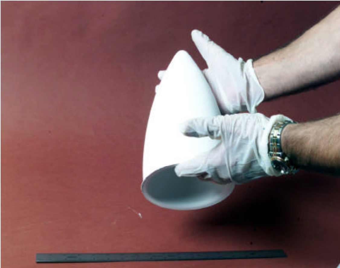
Figure 1: ALON dome as near net shape
