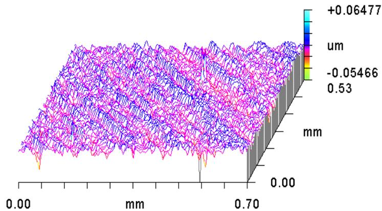
**Figure 6.** Phase plate surface finish results.
