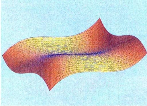
**Figure 4.** Surface of cubic phase plate.
