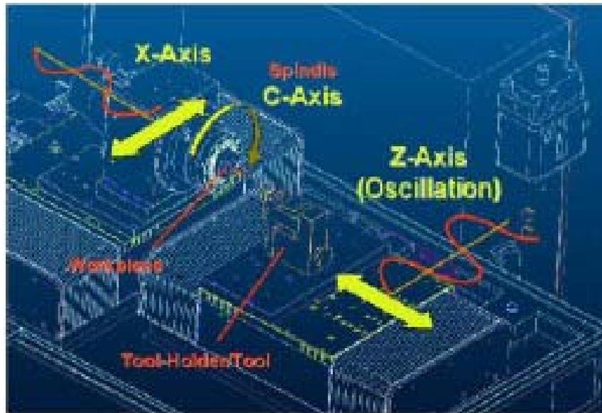
**Figure 3:** Set up with machining for Slow Slide Servo ( $S^3$ )
