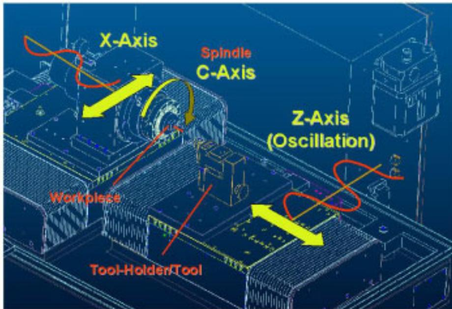
Figure 1: Setup for machining with Slow Slide Servo
