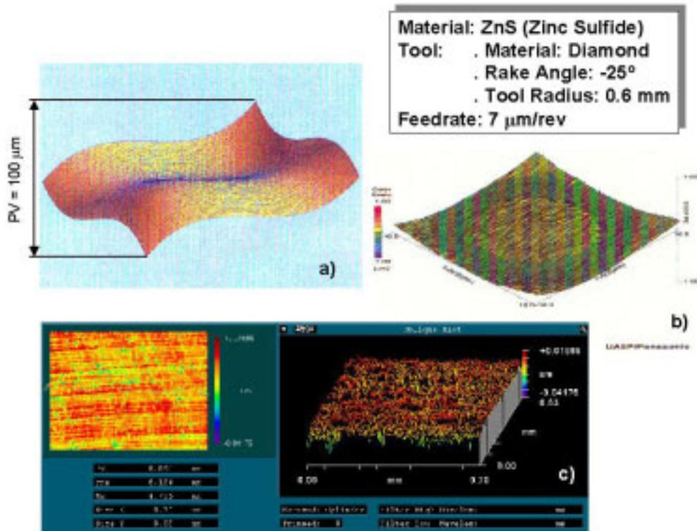
Figure 2: Cubic Phase Plate Surface. a) Mathematical representation of the cubic phase plate surface. b) Form accuracy measurement results (measured with Panasonic Profilometer UA3P). c) Surface finishing results (measured with Zygo NuView).
